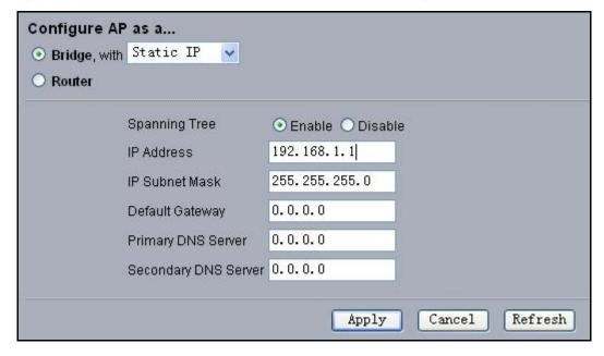
Figure 9 Configure the ZMAX-8210 to Bridge
